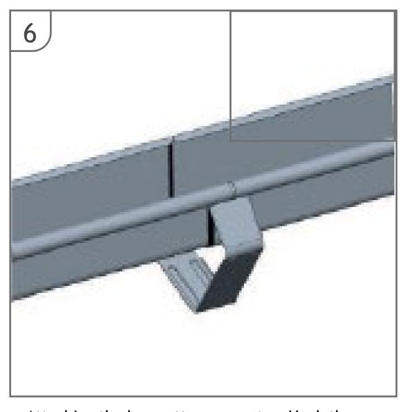
Attaching the box gutter connector: Hook the connector onto the bead at the front first, then pressing onto the adhesive surfaces of the seal throughout, wrap it around the gutter lengths over the join to the back.
