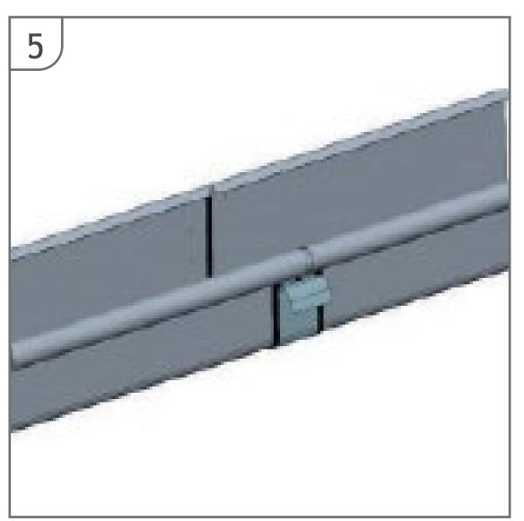
Remove the remaining protection film from the rubber sealing strip's final adhesive surface.
