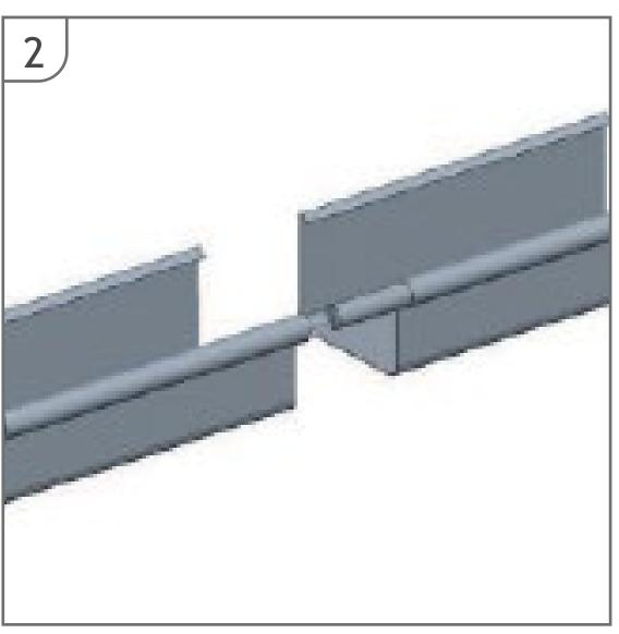
Insert the bead connector halfway into the front 'bead/rolls' of both gutters, leaving an approx. 5 mm gap between the ends of the two gutter lengths.
