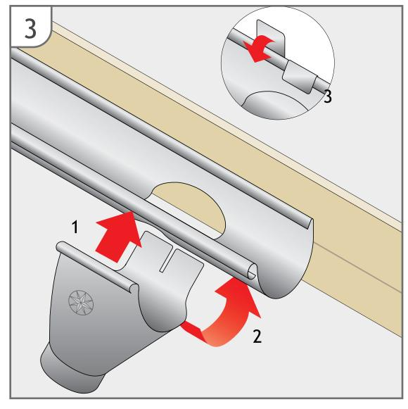
Attach the outlet to the gutter and fold the rear tabs of the outlet over the rear edge of the gutter, making sure the outlet is aligned correctly to accept the downpipe.
