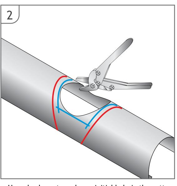
Use a hacksaw to make an initial hole in the gutter, and then use a set of tin snips to cut out the inner hole that you have marked out.
