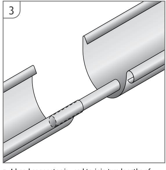
A bead connector is used to join two lengths of gutter. Insert the connector into the front roll of each gutter length. Allow for a 4mm expansion gap.
