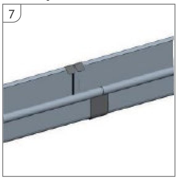
• Finally fold the flaps at tehe back of the connector over the rear fold of the gutter lengths.
