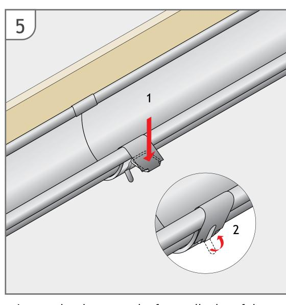
Locate the clasp over the front roll edge of the gutter. Push down on top of the clasp and squeeze the clasp shut. Fold the locking tab over to fully secure.
