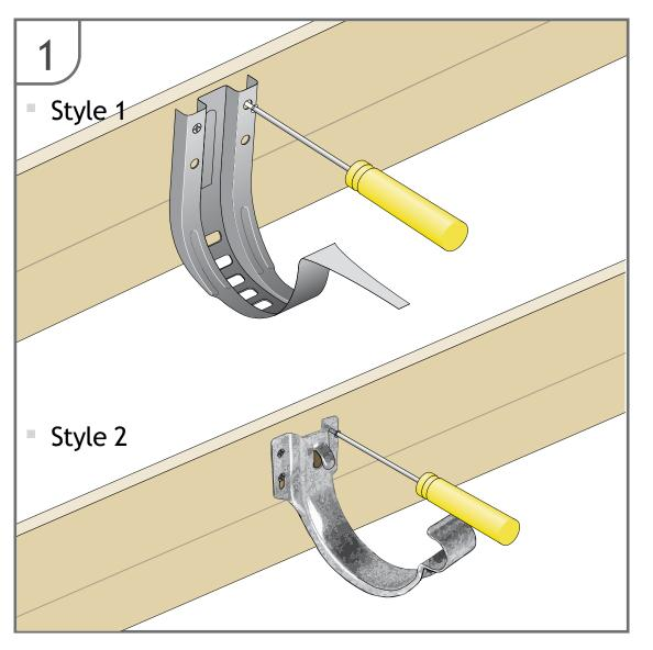
Generally position the fascia brackets at 915mm centres, using at least 3 brackets per gutter length.
