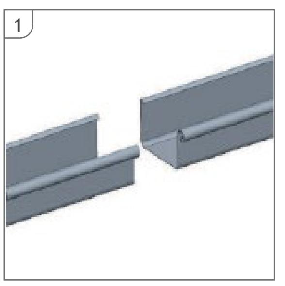
Clean the outer surfaces at the edges of both the lengths of gutter to be joined with a suitable cleaning agent (And if lengths have been cut down, deburr the ends).
