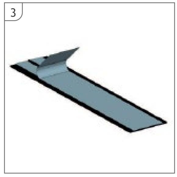
Remove the protection film from the adhesive surface (on ridged side) of the rubber sealing strip.
